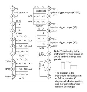
③ Thermocouples with different graduation numbers use different compensation wires for thermocouples. When using the internal automatic compensation mode, the compensation wires should be directly connected to the terminals on the back cover of the instrument, and cannot be converted into ordinary wires in the middle, otherwise measurement errors will occur.
