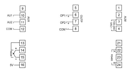
**Note 1**: 0~5V/1~5V and above voltage signals are input from 16+, 15-, 0~100mV and below signals are input from 14+, 15-; 4- 20mA linear current input and 250 ohm resistor into 1-5V, then input from 16+, 15-.
