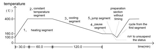
The advantage of using temperature-time programming method is that the slope setting range of temperature rise and drop is very wide. The heating and constant temperature sections have a unified setting format, which is convenient for learning. Besides, it is more flexible to set curve, and possible to set a continuous heating section (for example, use a heating section with different slopes to approximate functional heating), or a continuous constant temperature section as well.
