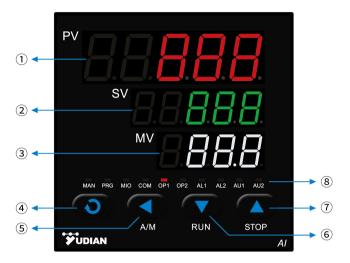
⑧10 LED indicator lights, MAN light on means in manual output state; PRG light on means in program running state, flashing in wait function state; The MIO, OP1, OP2, AL1, AL2, AU1, AU2 lights correspond to the input and output actions of the corresponding position module respectively; the COM light flashes to indicate that it is communicating with the upper computer.
