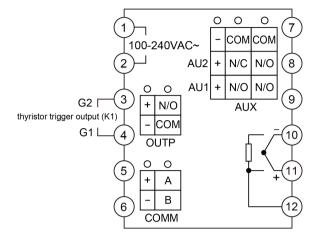
when the I2 module is installed and the bAud parameter is set to 1, the switch input function of the MIO module can be virtualized, the external switch on the 5th and 6th terminals
