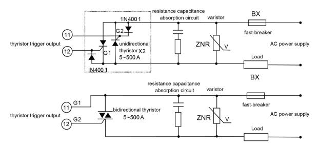
Note 1: Resistor-capacitor absorption and varistor must be added when phase-shift trigger is used to improve possible harmonic interference.
