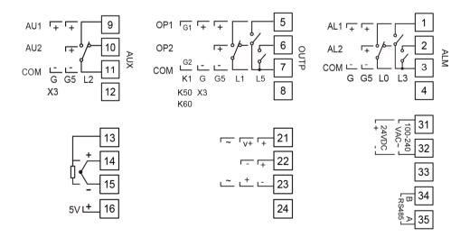
**Note 1**: 0~1V and above voltage signals are input from 16+, 15-, 0~100mV and below signals are input from 14+, 15-; 4-20mA linear current input and 250 ohm resistor into 1-5V, then input from 16+, 15-. Note 2:The main output module can choose G, X3, L2, K1, K50, K60, W1<sub>o</sub>
